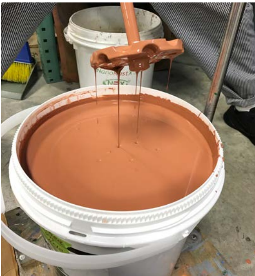
Use a mixing disc with a diameter of approximately 1/3 rd the diameter of the pail.
