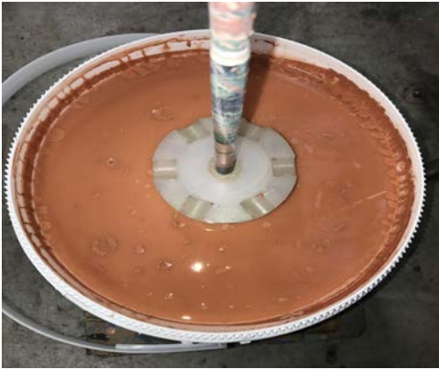
Use a mixing disc with a diameter of approximately 1/3 rd the diameter of the pail.
